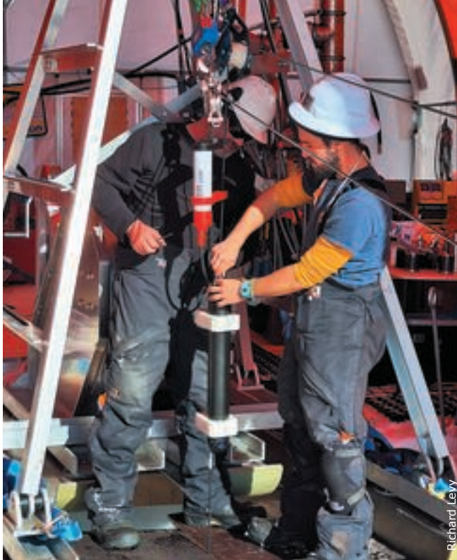
Martin (Paddy) Loughney (left) and Ollie Twigge (right) deploy an oceanographic mooring through a hole in the Ross Ice Shelf.
