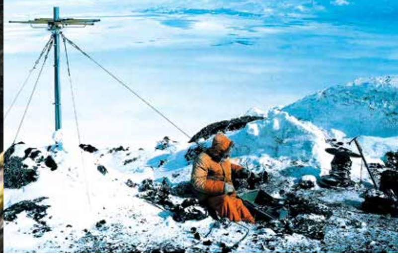
(6) Ray Dibble adjusting a seismometer transmitting to Scott Base
